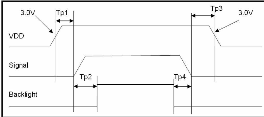
Figure 5.2 Interface power on/off sequenc
